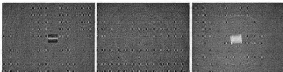
Figure 3. Growth inhibition of S. epidermidis ATCC 35989 on agar plates. (A) titanium, (B) PLGA 80/20, and (C) PLGA 80/20 containing ciprofloxacin. [Color figure can be viewed in the online issue, which is available at www.interscience.wiley.com .]
