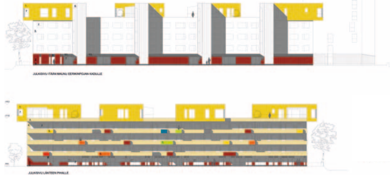
In the design the old prefab concrete balconies are replaced with a new wooden balcony belt the width of the entire facade. Small apartments will be constructed on the ground floor (old garage space). The town villas on the roof are a new, visible element.
