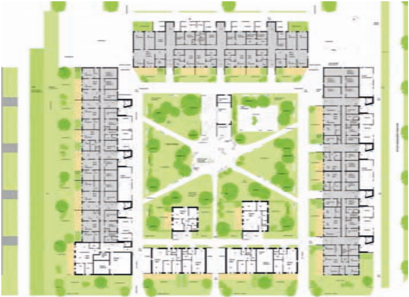
The courtyard will become private by nature because the low infill construction will close the block on the south side. The new buildings and new parts of the existing buildings are marked with white colour.
