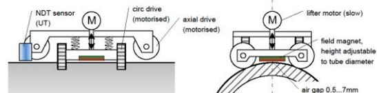
Magnetic attraction for stability on pipe, magnetic force modulation (varying air gap) for landing/take-off.
