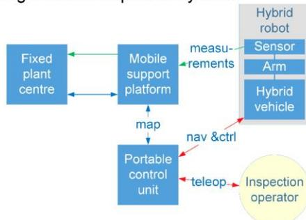
**Complete system**, including hybrid (flying and rolling) robot with robotic snake-arm, miniaturised ultrasonic sensor and a mobile operation support platform.
