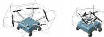
Tilted propellers for improved manoeuvrability plus assisting stability on the pipe (lateral thrust).
