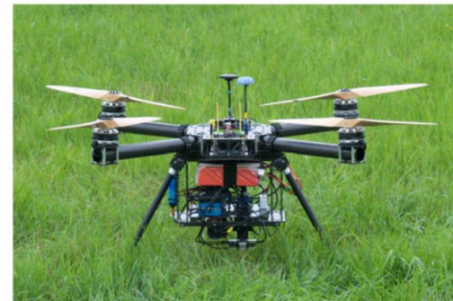
Figure 1 DroneKnowledge hyperspectral imaging system mounted under the Avartek drone.
