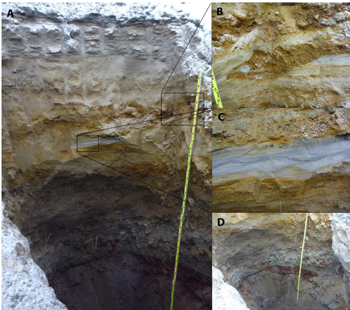
Fig. 17. Stratified sediment sequence under three metres thick till cover in Rantamaa sand pit, Liakka. Coarse core part composed of gravels is seen on the bottom (A, D). Upper parts include cross and planar bedded sands with gravelly or silty interlayers. Some catchment/injection structures (B) and ripple marks (C). Photos by P. Sarala.
