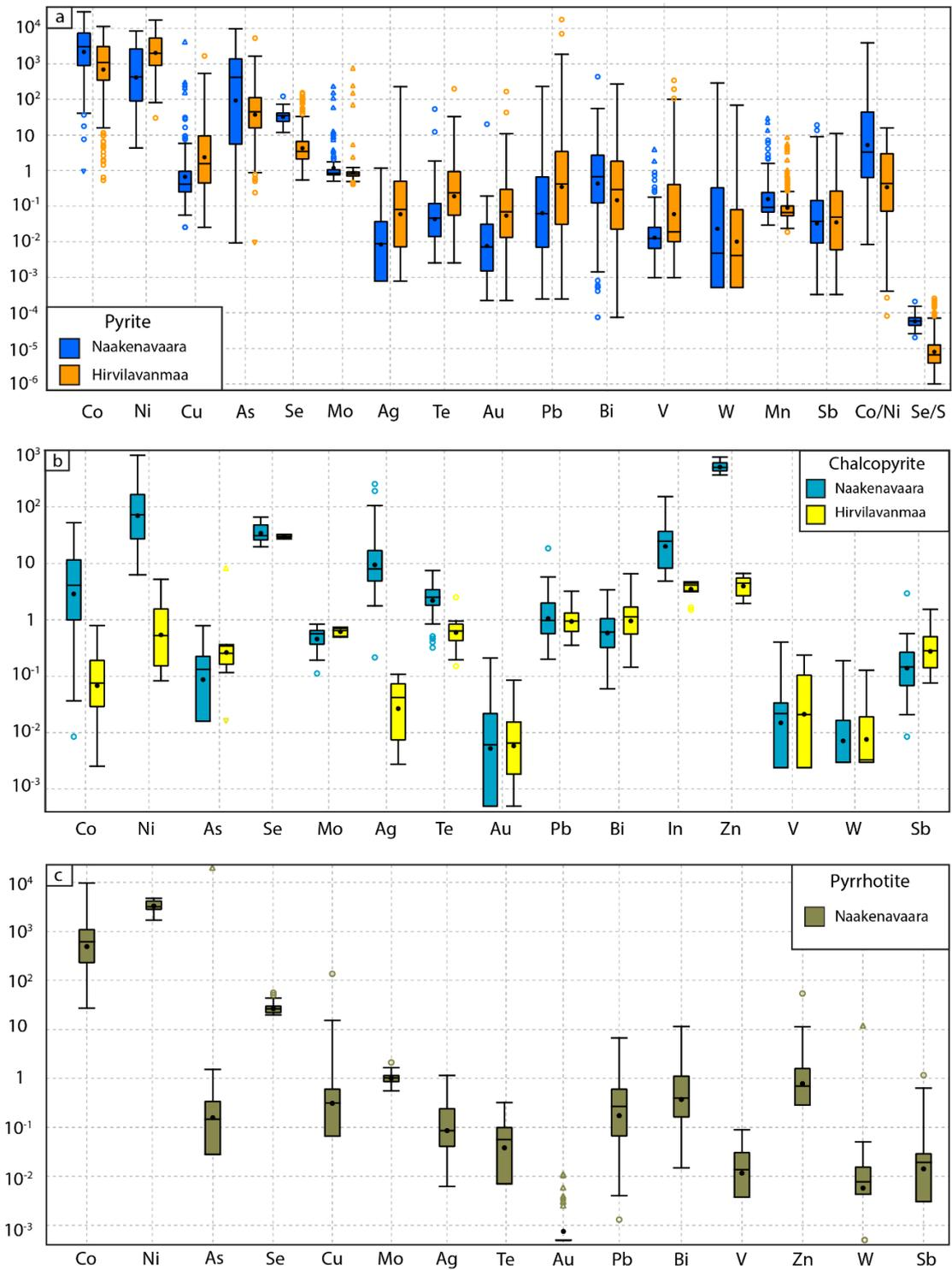
**Figure 6.** (a) Selected trace element boxplots with logarithmic scale for pyrite from Hirvilavanmaa (orange boxes) and Naakenavaara (blue boxes). (b) Selected trace element boxplots with logarithmic scale for chalcopyrite from Hirvilavanmaa (yellow boxes) and Naakenavaara (light blue boxes). (c) Selected trace element boxplots with logarithmic scale for pyrrhotite from Naakenavaara. Figure taken from Vasilopoulos et al. (2023).
