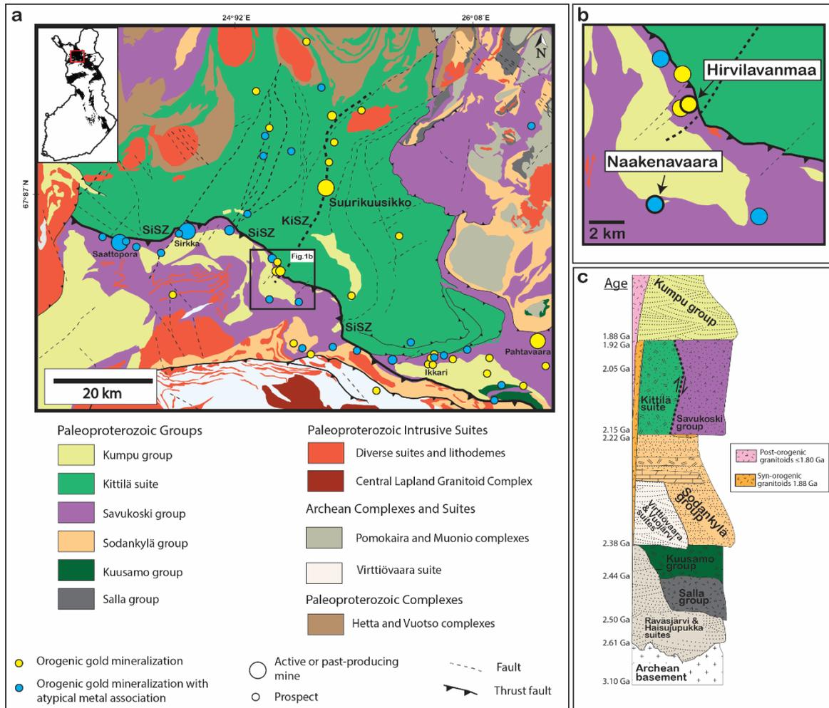
**Figure 1.** (a) Simplified geological map of Central Lapland belt (CLB) showing location of discovered Au-only (yellow circles) and atypical base metal-rich (blue circles) orogenic Au deposits and occurrences. Inset map shows the position of CLB in Finland. (b) Detailed view of marked area from Fig. 1a, showing location of the Hirvilavanmaa and Naakenavaara deposits. (c) Stratigraphic column of CLB, modified after Köykkä et al. (2019). Figure taken from Vasilopoulos et al. (2023)
