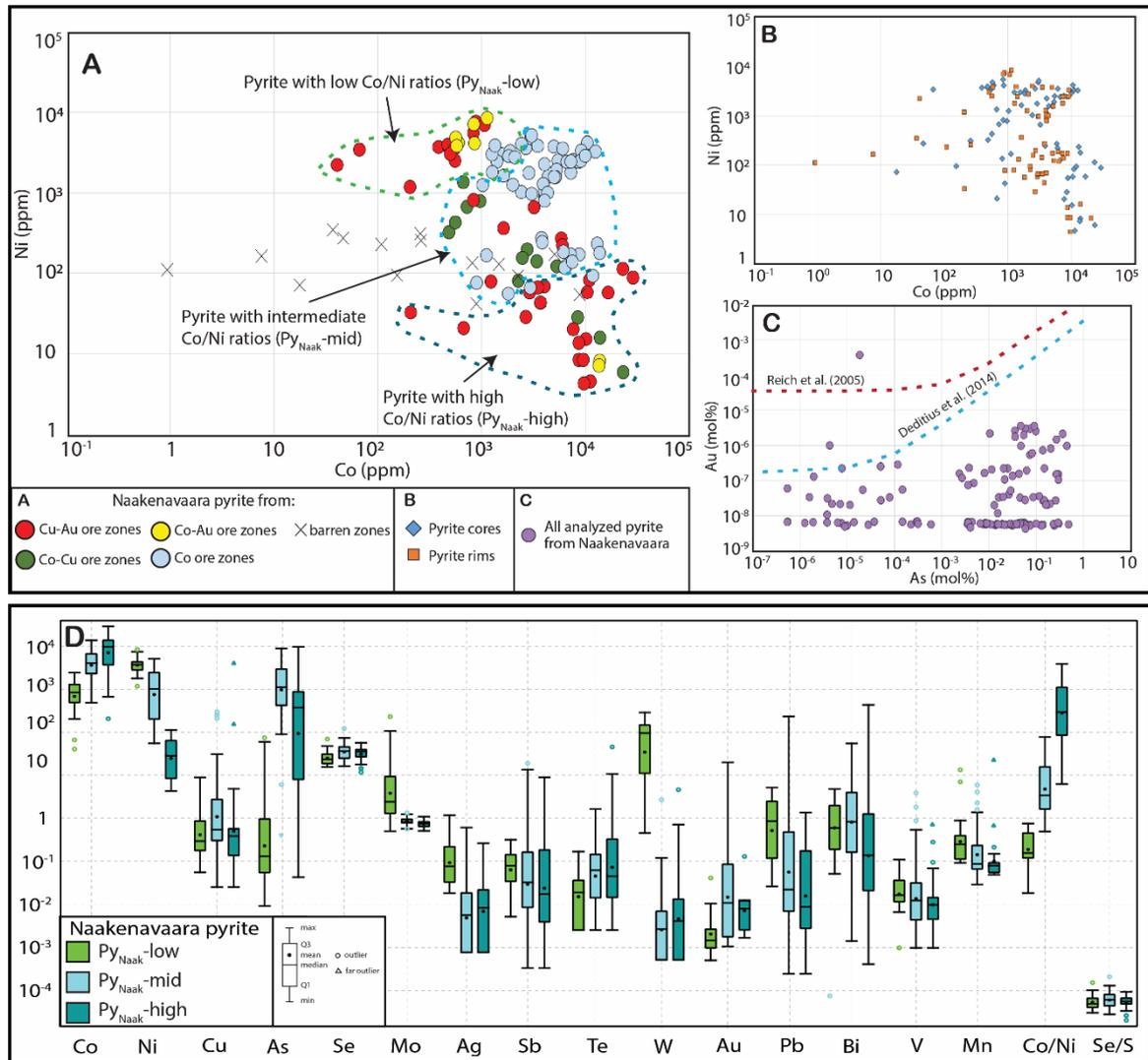
**Figure 8.** (A) Co-Ni plot for Naakenavaara pyrite with data points classified according to degree of Au enrichment in the samples. (B) Co-Ni plot for Naakenavaara pyrite with data points classified based on a core-rim distinction. (C) As-Au plot for Naakenavaara pyrite with Au solubility lines from Reich et al. (2005) and Deditius et al. (2014). (D) Trace element boxplots with logarithmic scale for the different types of pyrite from Naakenavaara. Figure taken from Vasilopoulos et al. (2023)
