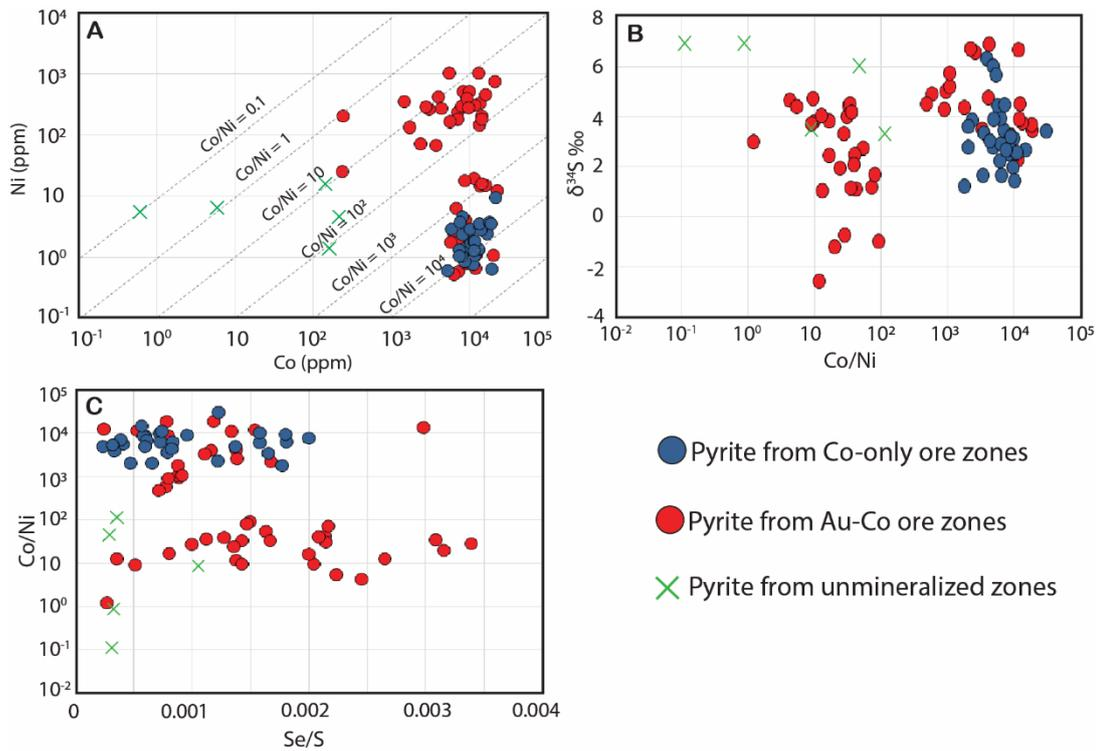
**Figure 5.** (A) Co vs. Ni scatterplot diagram for pyrite from Juomasuo. Lower cluster with high Co/Ni ratios includes pyrite associated with chlorite and deposited during the Co-rich stage. Pyrite in the upper cluster includes pyrite associated with sericite and deposited during the subsequent Au-rich stage. (B) Co/Ni vs.  $\delta^{34}\text{S}$  scatterplot diagram for pyrite from Juomasuo. Figure modified from Vasilopoulos et al. (2021)
