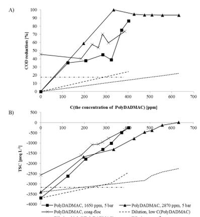
Fig. 3. A) COD reductions and B) development of TSC values for DAF studies with *PolyDADMAC* for O/W emulsions.
