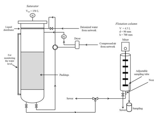
Fig. 2. DAF set-up
