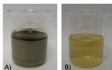
Fig. 1. Real oily wastewater A) before and B) after UF treatment.
