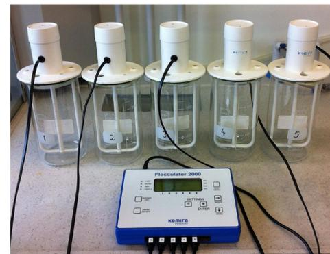
Fig. 1. The jar test device Kemira Kemwater Flocculator 2000.
