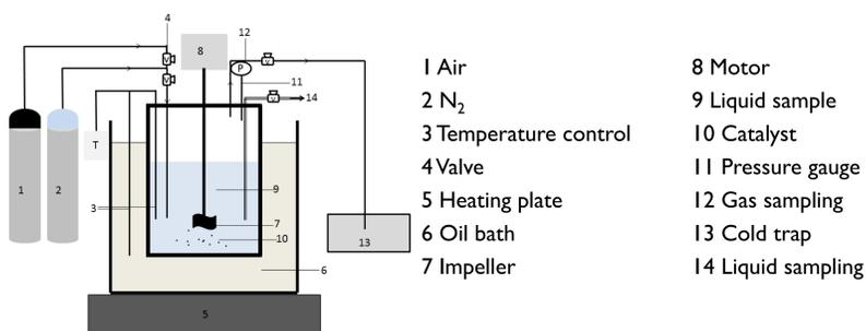
Fig. 1. Schematic diagram of the CWAO experimental set-up.
