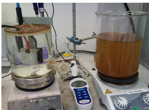
Fig. 1. Peat bog drainage water before and after EC-treatment (approx. operating costs 0,2 €/m<sup>3</sup> & treatment time 15 min).
