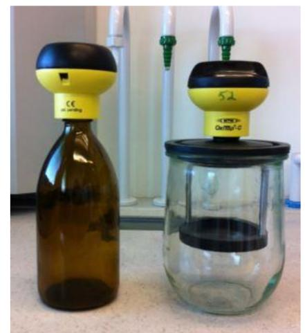
Fig. 1. OxiTop measuring system for liquid and solid measurements.
