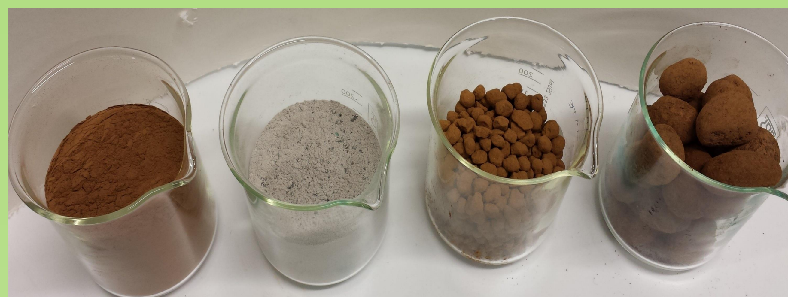
Fig. 3. From left to right: bio-ash, steel slag and small- and large-sized symbiosis pellets containing bio-ash and steel slag.
