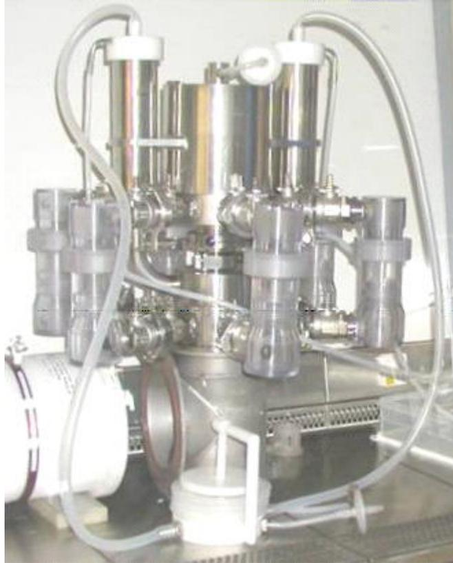
Fig. 5: The Leeds six-station pulsatile flow heart valve bioreactor.
