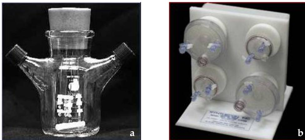
Fig. 2: a) Spinner flask bioreactor, b) Synthecon® rotating wall vessel bioreactor.
