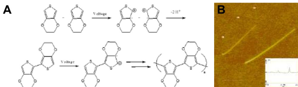
**Figure 3.** (A) Scheme for the oxidative polymerization mechanism of poly-EDOT. (B) Two poly-EDOT lines written with speed of 10 (left) and 1 nm/s (right). Line width: 50 nm. Inset: Cross-section of the two lines. (Reproduced with permission from Ref. 33)
