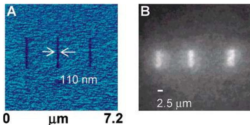
**Figure 2.** (A) Lateral force microscopy (LFM) image of 2- $\mu\text{m}$ -long lines of MPTMS written by DPN on glass. (B) Fluorescent image of three 2.5  $\mu\text{m}$   $\times$  10  $\mu\text{m}$  regions of MPTMS conjugated with biotin-maleimide and Cy3-streptavidin. (Reproduced with permission from Ref. 28)
