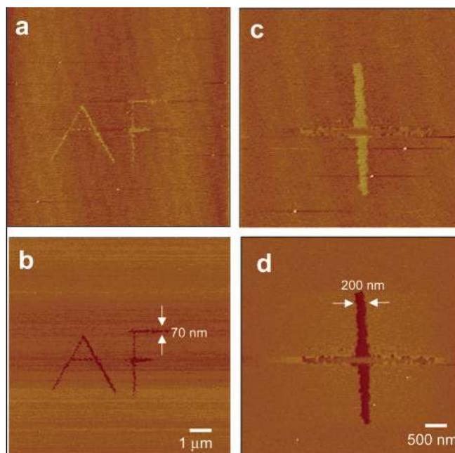
**Figure 4.** Nanoscale patterns written with the peptide MH2 on a gold surface using TappingMode DPN. (a) Height image of “AF” written using an aspect ratio of 1: 64 and various scan angles. The corresponding phase image (b) shows a darkened patterned region. (c) Height and (d) phase image of “+” written with aspect ratio of 1:32. Line widths of patterns are indicated. (Reproduced with permission from Ref. 51).
