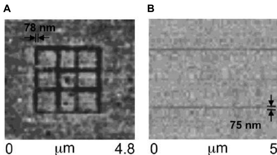
**Figure 1.** Lateral force microscopy (LFM) images of DPN-generated TMS monolayer patterns on semiconductor surfaces. (A) TMS grid on Si/SiO<sub>x</sub> substrate (2.4 μm edge width) and (B) a parallel line pattern on oxidized GaAs. (Reproduced with permission from Ref. 9)
