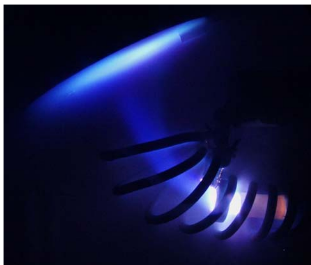
A carbon-polymer arc discharge. The ring shaped anode can be seen on the right, the sample is on the left.
