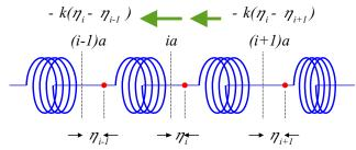
We consider N identical particles coupled to each other by identical parallel springs. The Lagrangian of the system is
